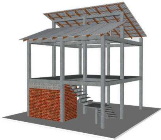
*Image 5 - A housing base, approx. 8,200 USD. The option comprises the structure, roofing, kitchen, and the clean and waste water systems © The Room Studio.*
